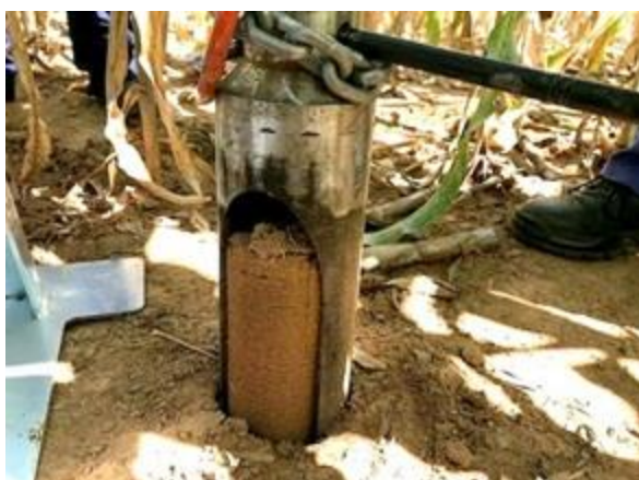
Figure 8 : Core sampling with GPS position
