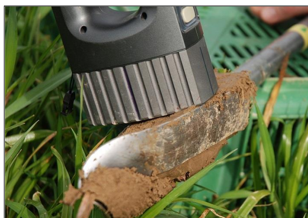
Figure 9 : Measurement with a visible near infrared spectrometer (VIS-NIR)
